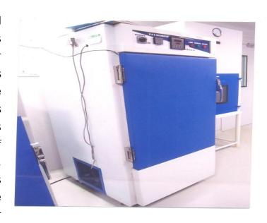
closed on a resilient gasket and permits inspection of stores without disturbing the same. Lock and key arrangements is provided in the double walled outer door, also fitted a door operated lamp for illumination inside the chamber. The unit is mounted on caster wheels for ease of mobility.
